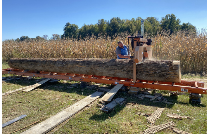
At the sawmill, turning a tree into lumber for the 19-foot-long-throwing arm
