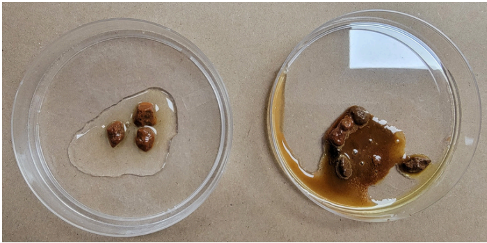
In acid tests, the brick samples (left) were not affected by muriatic acid, while the daub (right) was dissolved by the acid.
