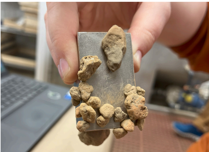
Magnet test showing that the pre-European-contact-period daub found at the boarding house excavation was magnetic. Brick found at the same site was not attracted to the magnet. .
